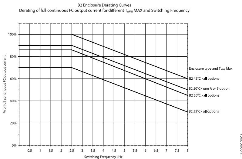
Illustration 1.12: B2 Enclosure Derating Curves. Derating of full continuous FC output current for different T<sub>AMB</sub> MAX and Switching Frequency
