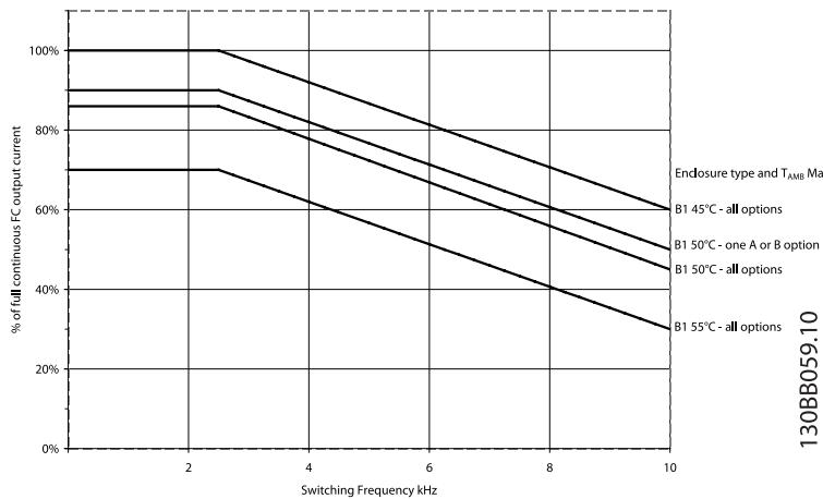
Illustration 1.11: B1 Enclosure Derating Curves. Derating of full continuous FC output current for different T<sub>AMB</sub> MAX and Switching Frequency
